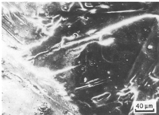
Figure 3 Slight pitting (bubbles start to form) on the surface of SiC after corrosion in the V_2O_5 melt for 2 h at 1000^\circ C .
